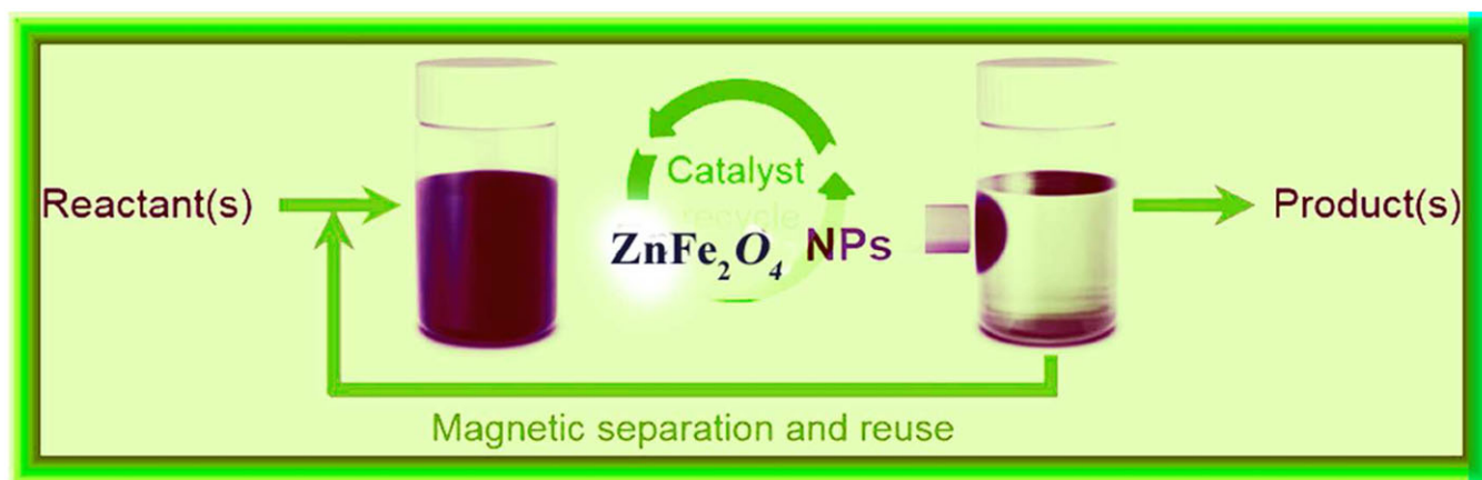
SCHEME 3 Separation of catalyst ( \text{ZnFe}_2\text{O}_4 ) from reaction mixture using an external magnet
